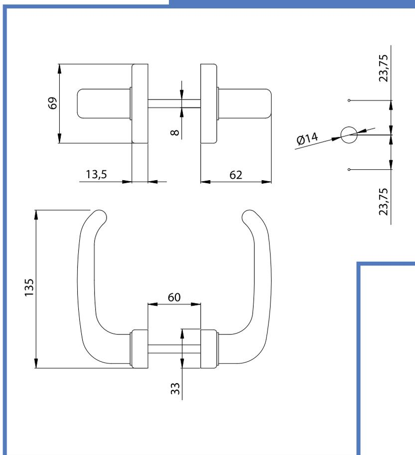
Double handle in nylon with return spring for fitment onto door pillar or central door strip. Fitted with a mechanism that guarantees a valid support to the lock's spring in keeping the handle horizontal.
